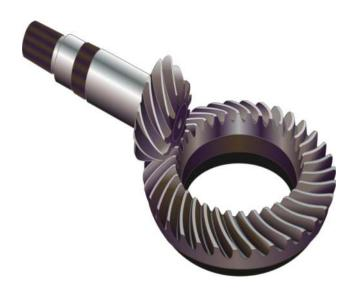
A bevel gear is shaped like a right circular cone with most of its tip cut off. When two bevel gears mesh, their imaginary vertices must occupy the same point. Their shaft axes also intersect at this point, forming an arbitrary non-straight angle between the shafts. The angle between the shafts can be anything except zero or 180 degrees. Bevel gears with equal numbers of teeth and shaft axes at 90 degrees are called miter gears.
